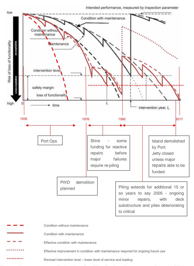
Figure 1 How we got here - Tanker Jetty Condition (Ageing of a structure – (sources CIRIA C674 & The Rock Manual  $^8$ )
