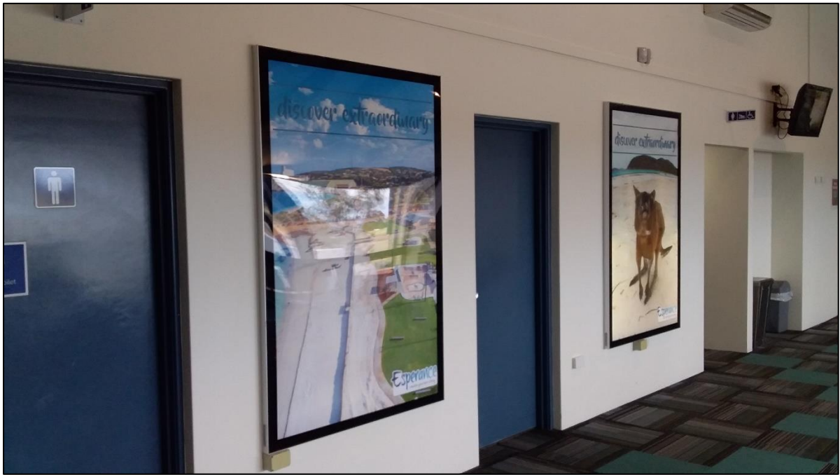
Figure 4: Signage locations 6 and 7, non-cycling rear illuminated fixed advertisements measuring approximately 1200 x 1800mm (1120 x 1710mm internal) each. Rear illuminated 'light box' signs need to be printed in standard light box GSM backlit polypropylene.
