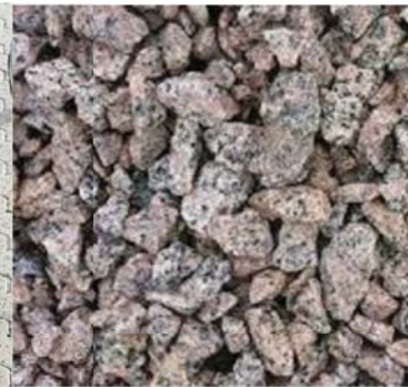
CRUSHED LOCAL GRANITE FOR DRAINAGE VOIDS IN PERMEABLE PAVING. (AGGREGATE SIZE 2-5mm)
