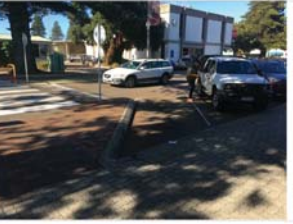
DEMPSTER STREET CROSS OVER NEAR ANDREW STREET: THE PATH OF TRAVEL FOR PEDESTRIAN IS CUT OF BY THE PROXIMITY OF ANGLED PARKING. PEDESTRIANS OFTEN CUT THROUGH THIS PARKING BAY AND ARE AT RISK OF BEING INJURED BY CARS PULLING IN BEHIND OR IN FRONT OF THEM.
