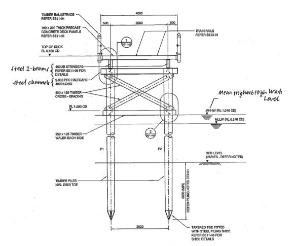
TYPICAL PIER ELEVATION - TIMBER PILES
