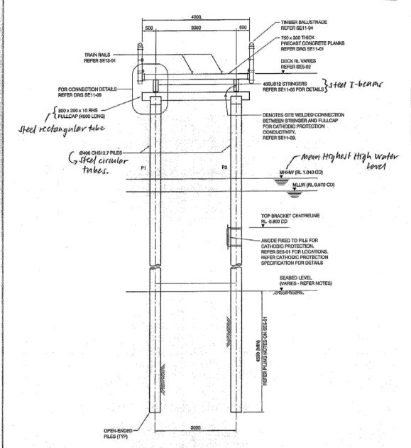
TYPICAL PIER ELEVATION - STEEL PILES
